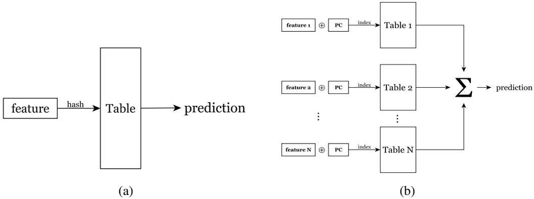
Fig. 2. (a) Previous PC-based Reuse Predictors and (b) Perceptron-based Reuse Predictor
