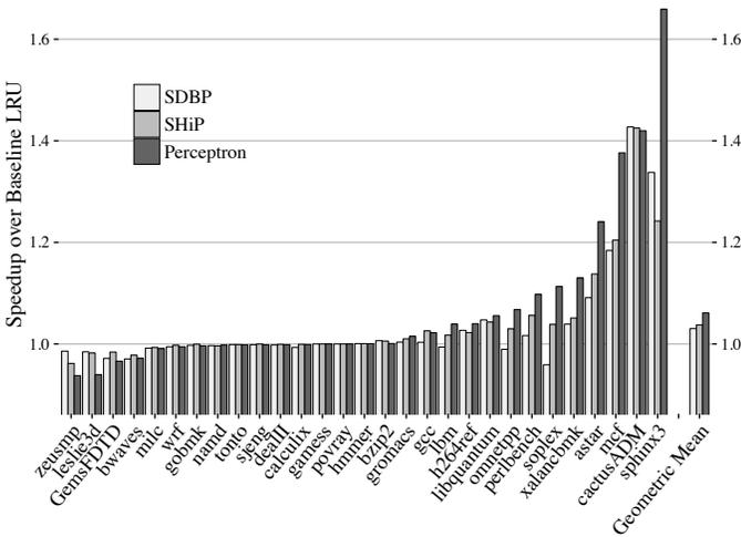
Fig. 7. Speedup over LRU for Single-Thread Workloads.
